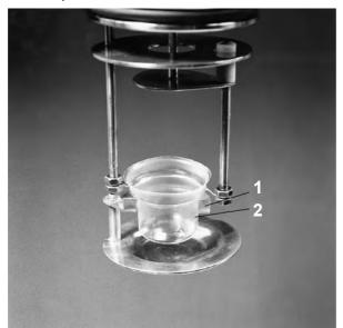
Placing the combustible crucible Crucible holder (part of C 5010.4) (not in scope of supply) Combustible crucible (not in scope of supply)
